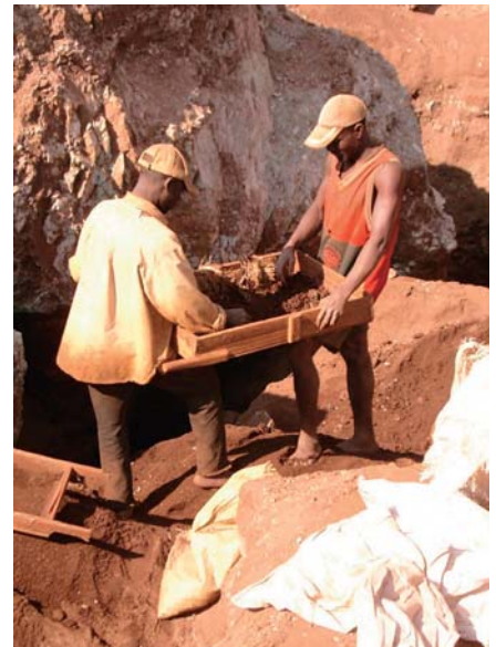
Young 'cresseurs' screening copper/cobalt oxide ore at the Luputo artisanal mine near Kipushi, Katanga, Democratic Republic of Congo
